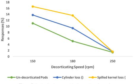
Figure 7: Evaluation Losses at 5 kg Peanut Kernel quantity
