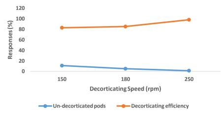
Figure 6: Evaluation at 5 kg Peanut Kernel quantity and decorticator efficiency
