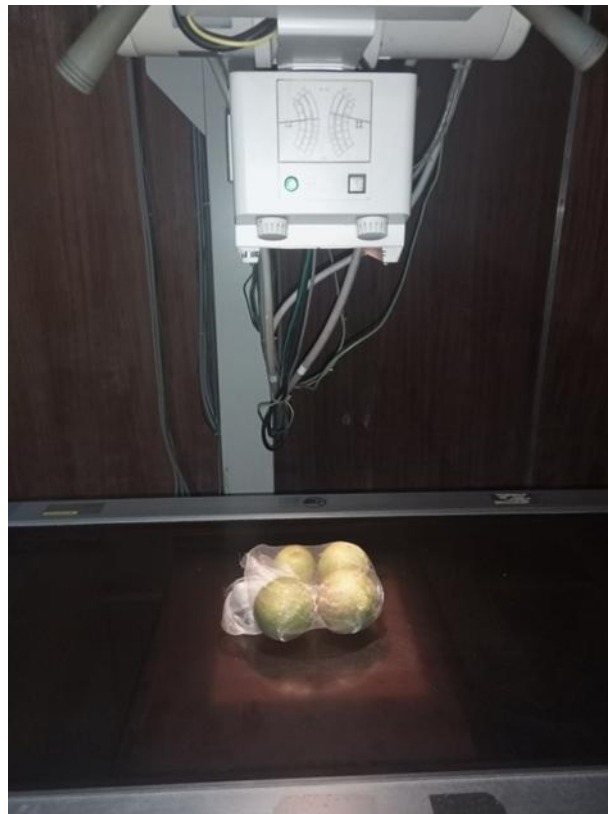
Fig 1 Setup of the X-ray exposure of orange fruits
