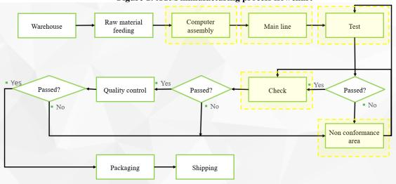
Figure 1: ATM manufacturing process flowchart
