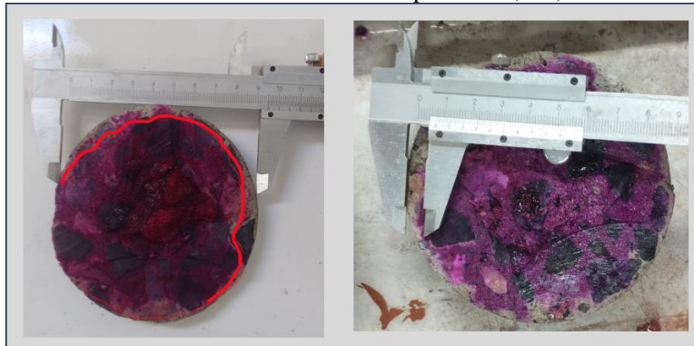
Figure 2: Measurement Scheme Extracted from Test Specimens (TSs) via Circular Saw Cutting 7 .
