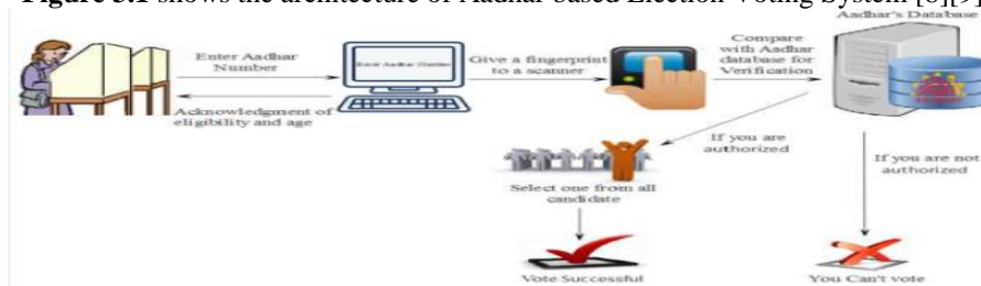
Fig 3.1: Architecture of Aadhar based Election Voting System
