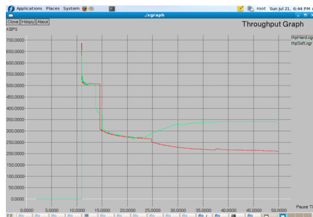
Fig. 2: Throughput for Hard Wimax and Soft Wimax
