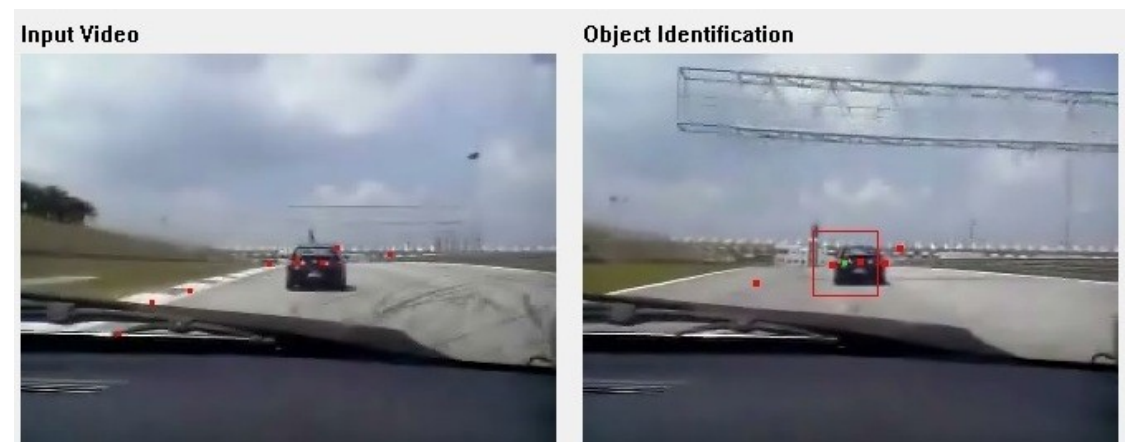
Fig 6: Automatic Identification of Object using Trajkovic-4 Corner Detector
