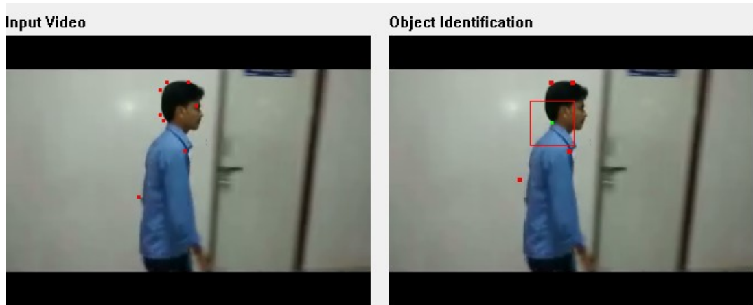
Fig 7: Automatic Identification of Object using Trajkovic-8 Corner Detector
