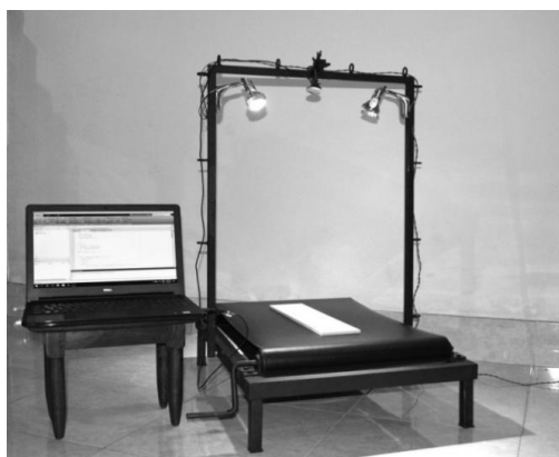
Fig.9. Developed electronic eye cut tile measuring function
