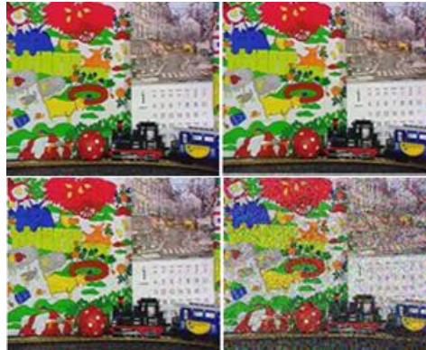
Fig. 3 : A frame of mobile & calendar with additif gaussian white noise : de left to right : original (from EPFL DB [11]); blurred with \sigma = 0,001 ; 0 ,01 et 0,1 respectively
