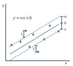
Figure 2. Linear regression with the epsilon range. Source: Data Mining Map https://www.saedsayad.com/ support\_vector\_machine\_reg.htm
