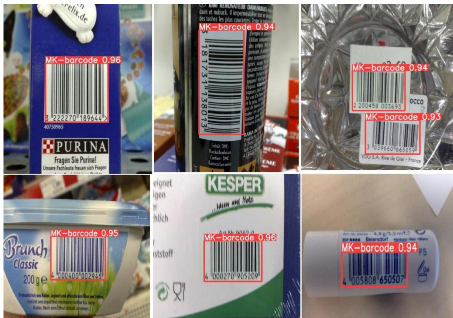
Figure 1 Samples of the utilized datasets where the YOLO-v5 successfully identified the barcode.
