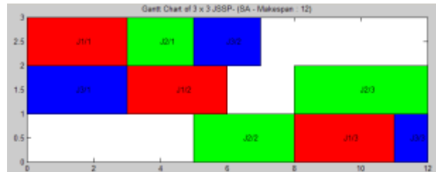
Figure 2 : The Gantt-Chart Representation of the Solutions found by SA based algorithm for the previously mentioned 3x3 Problem
