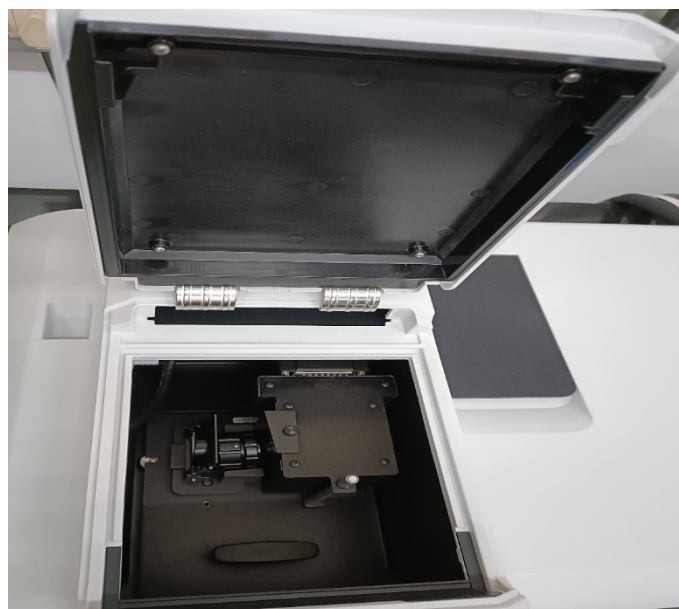
FIGURE 17- TOP LOADING TRAY MECHANISM
