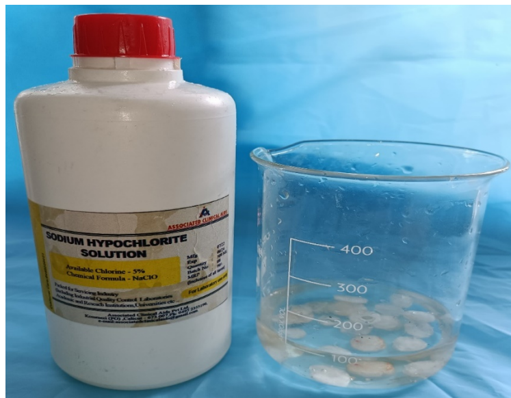
FIGURE 4- SAMPLES IMMERSSED IN 5.25% SODIUM HYPOCHLORITE
