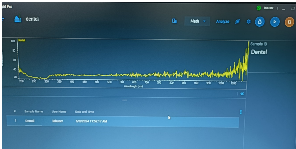
FIGURE 19- COLOUR STABILITY READING OF THE SAMPLE FROM WHITE COLOUR.
