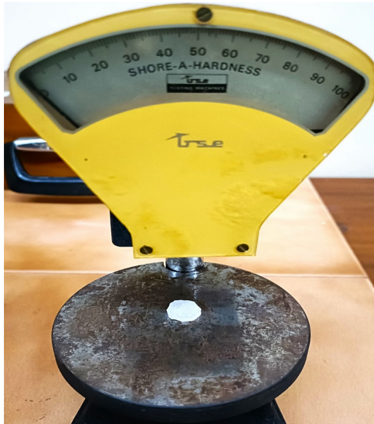
FIGURE 14- SAMPLE IS PLACED IN THE PLATFORM TO TEST THE SURFACE HARDNESS
