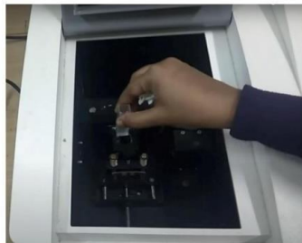
Sample being placed in the spectrophotometric machine to check the release of CHX from the solution.
