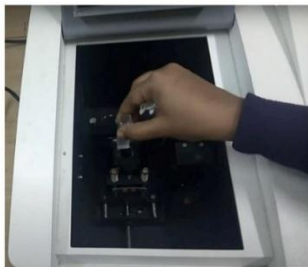
Sample being placed in the spectrophotometric machine to check the release of CTIX from the solution.
