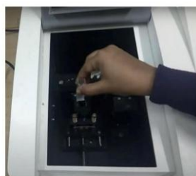
Sample being placed in the spectrophotometric machine to check the release of CHX from the solution.
