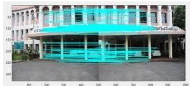
Fig -11: Feature Extracted Using SIFT
