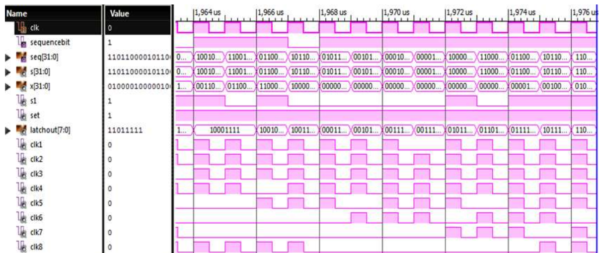
Fig.4.2. Simulation waveforms of an LFSR with Data-Driven clock gating
