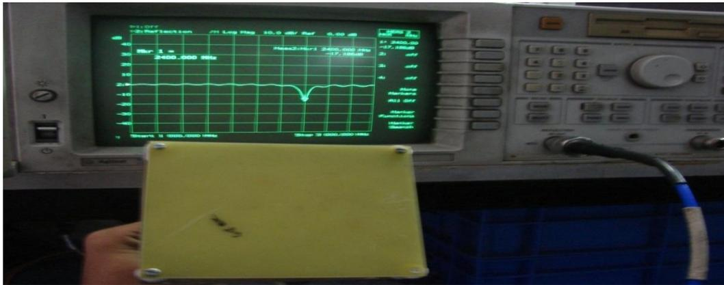
**Fig.5** Measurement set up for fabricated microstrip patch antenna with dielectric superstrate for measurement of return loss
