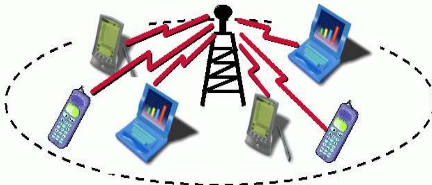
Fig.1 In this fig we can see there is one base station, through which all the devices like mobiles and laptops are connected. Base station transfers the data to all devices.
