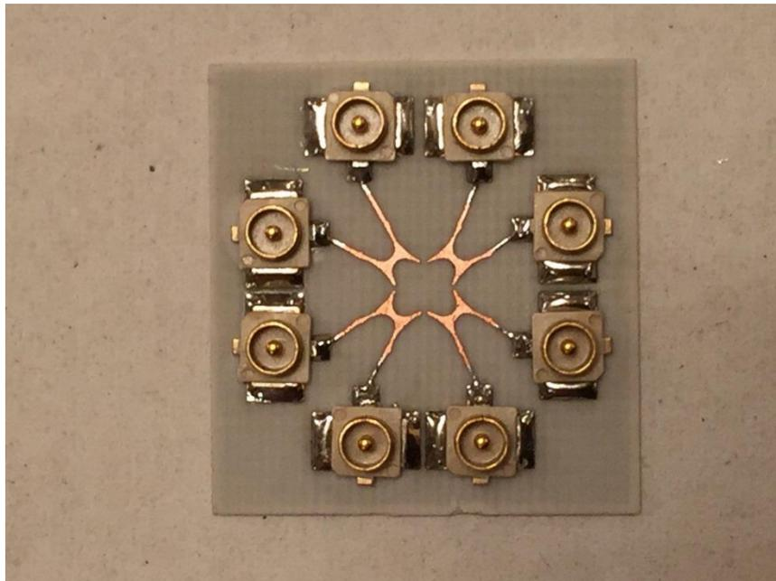
**Figure 1b.** The photograph of the proposed of Nnovel Ultra Broad-Band Exponential Taper Transmission Line 8- Port Network
