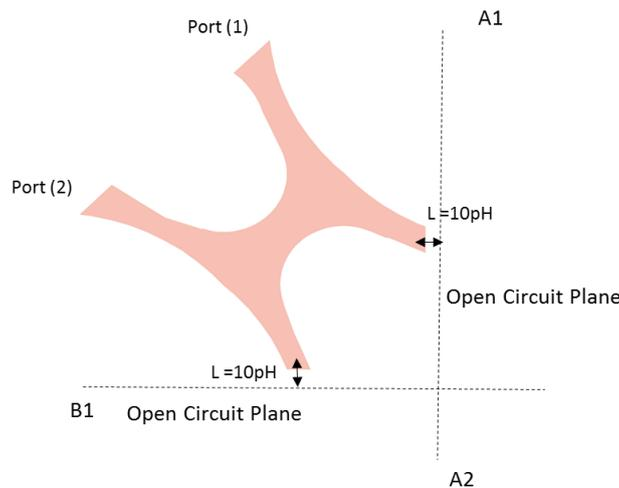
**Figure 2** shows the even-even mode equivalent circuit of figure 1 i.e. both planes A1 A2 and B1 B2 are having magnetic walls properties
