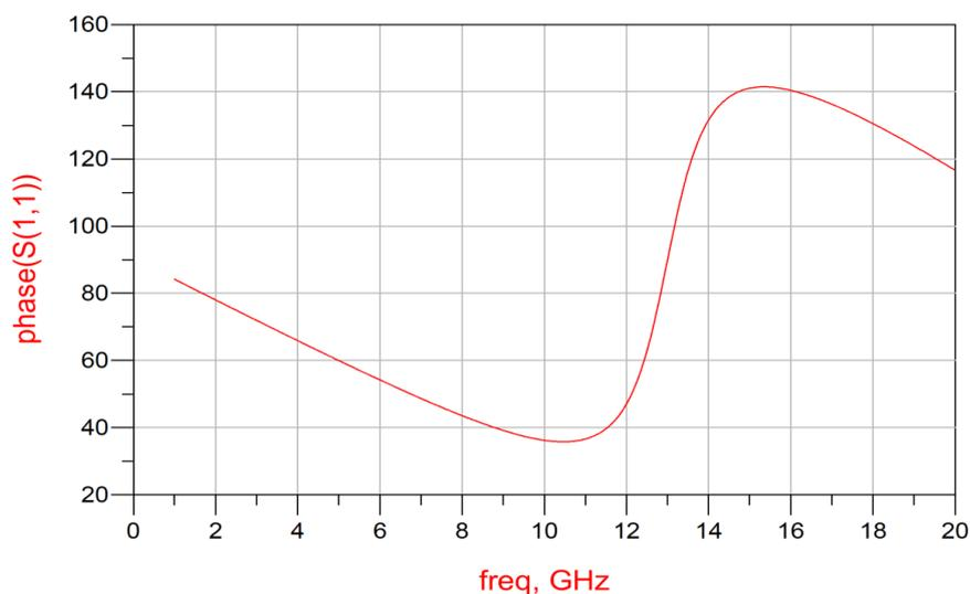
**Figure 6c.** The frequency responses of the Novel Ultra Broad-Band Exponential Taper 8-Port network in phase
