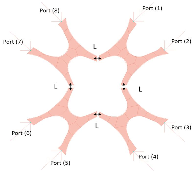
**Figure 1a** shows the layout of the Novel Ultra Broad-Band Exponential Taper Transmission Line 8- Port Network
