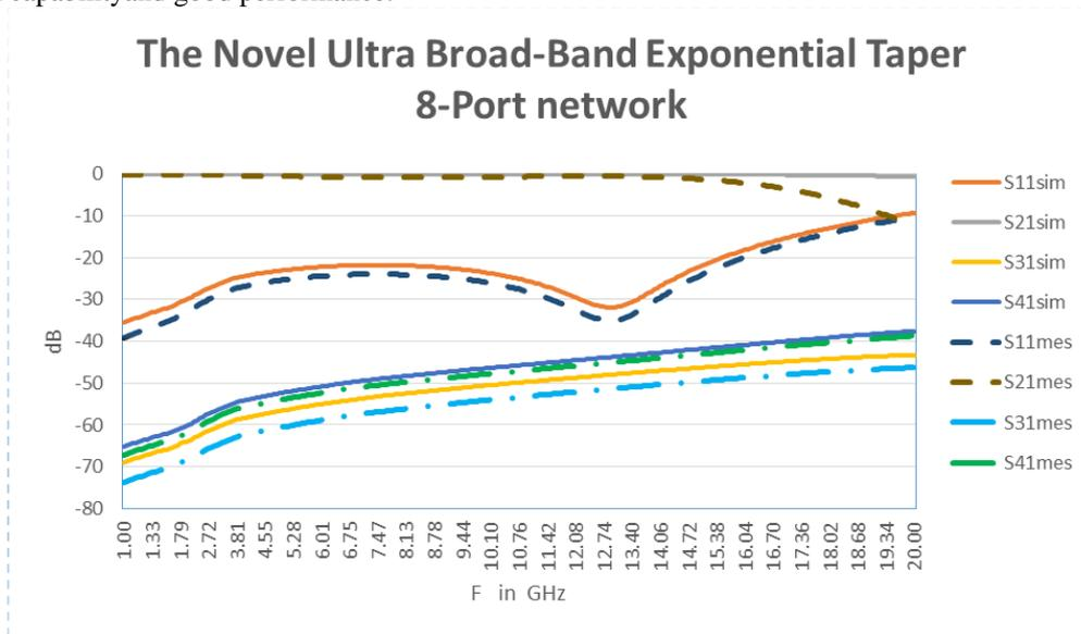
**Figure 6a.** The frequency responses of the Novel Ultra Broad-Band Exponential Taper 8-Port network
