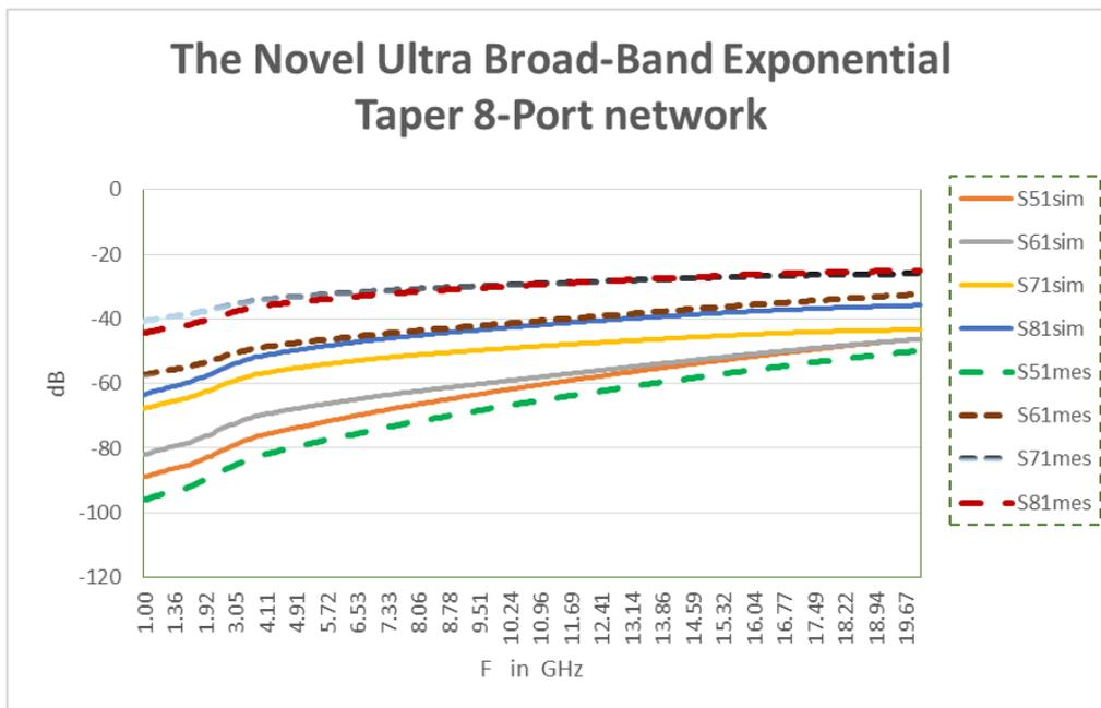
**Figure 6b.** The frequency responses of the Novel Ultra Broad-Band Exponential Taper 8-Port network
