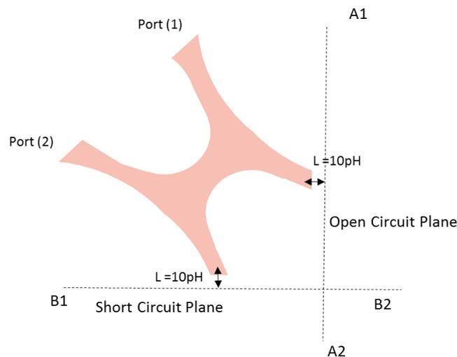
**Figure 3** shows the even-odd mode equivalent circuit of figure 1 i.e. both planes A1 A2 unopened circuit property (even mode) while plane B1 B2 is having short circuit property (odd mode property)
