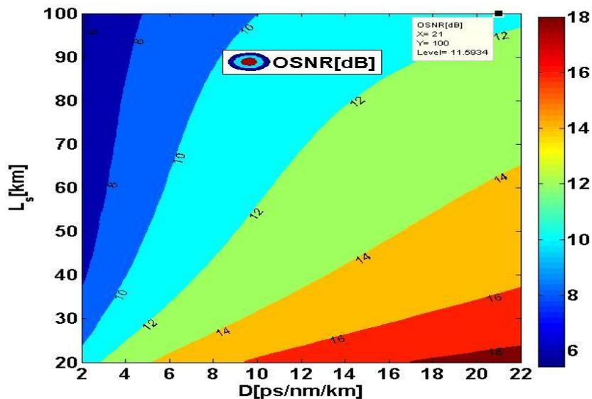
Fig.4. (a): Considering line rate 16GBaud, contour plot of OSNR versus span length [km] and dispersion [ps/nm/km] parameter of SF.
