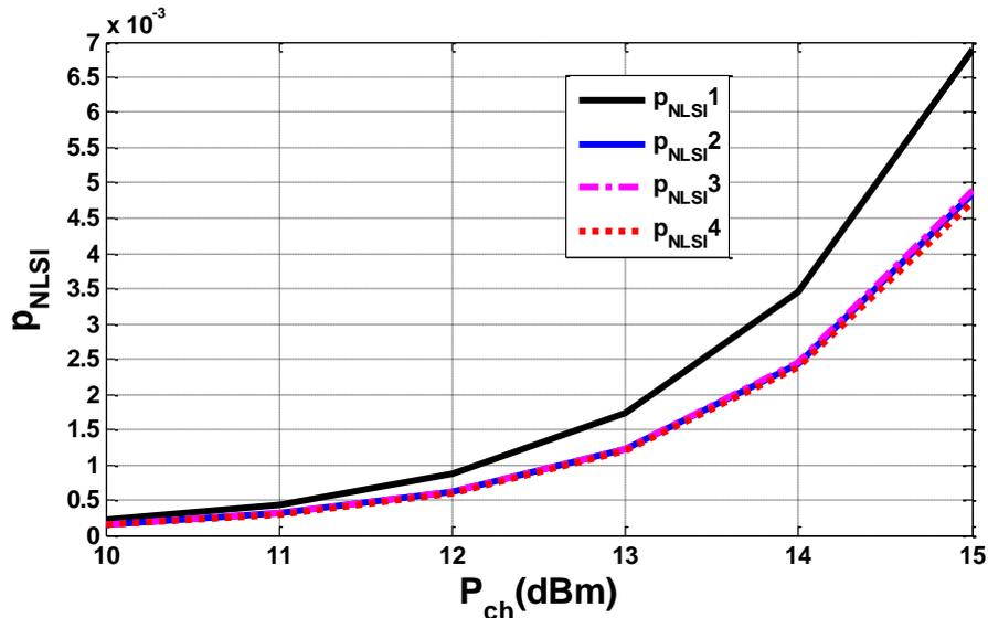
Fig. 2 (b): Non-linear signal interference for four GN models considering power of nonlinear signal interference ( $P_{NLSI}$ ) vs. channel power ( $P_{ch}$ ) with SF.
