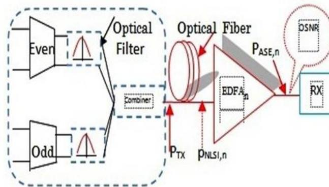
Fig. 1: Model of optical link.
