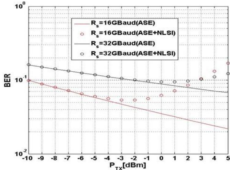
Fig.3. (b):  $P_{TX}$  [dBm] versus BER based on linear and nonlinear propagation considering 16GBaud and 32GBaud line rates of the COTS of SF
