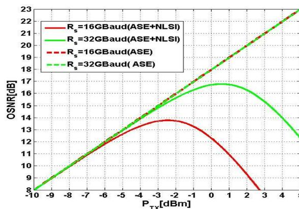
**Fig.3. (a):** OSNR [dB] versus  $P_{TX}$  [dBm] based on linear and nonlinear propagation considering 16GBaud and 32GBaud line rates of the COTS of SF
