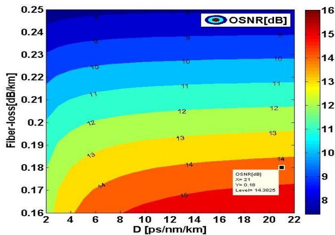
Fig. 4(d): Considering line rate 32GBaud, contour plot of OSNR [dB] versus fibre loss coefficient [dB/km] and dispersion [ps/nm/km] parameter for SF
