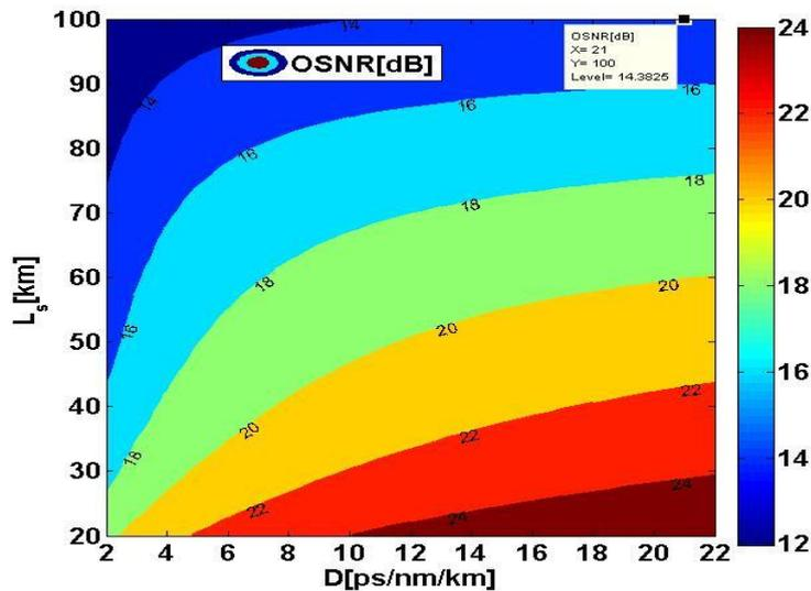
Fig. 4. (c): Considering line rate 32GBaud, contour plot of OSNR [dB] versus span length [km] and dispersion [ps/nm/km] parameter of SF
