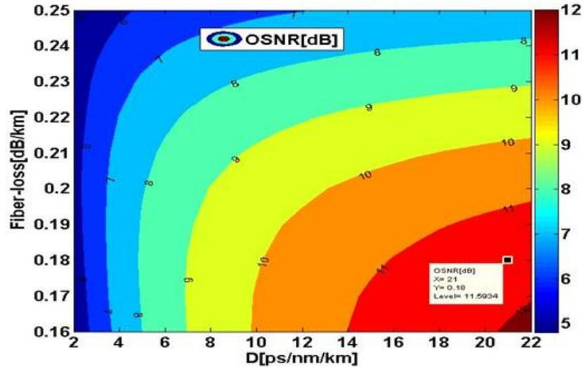
Fig. 4(b): allowing for line rate 16GBaud, contour plot of OSNR [dB] versus fibre loss [dB/km] and dispersion [ps/nm/km] parameter of SF
