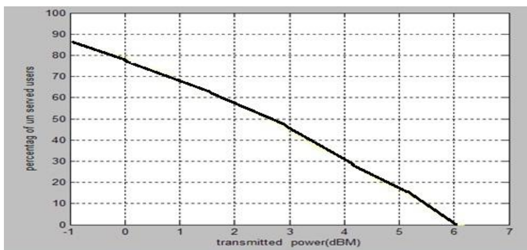
Fig-3 Transmitted Power (dbm) Vs percentage of un-served users shows the inverse
