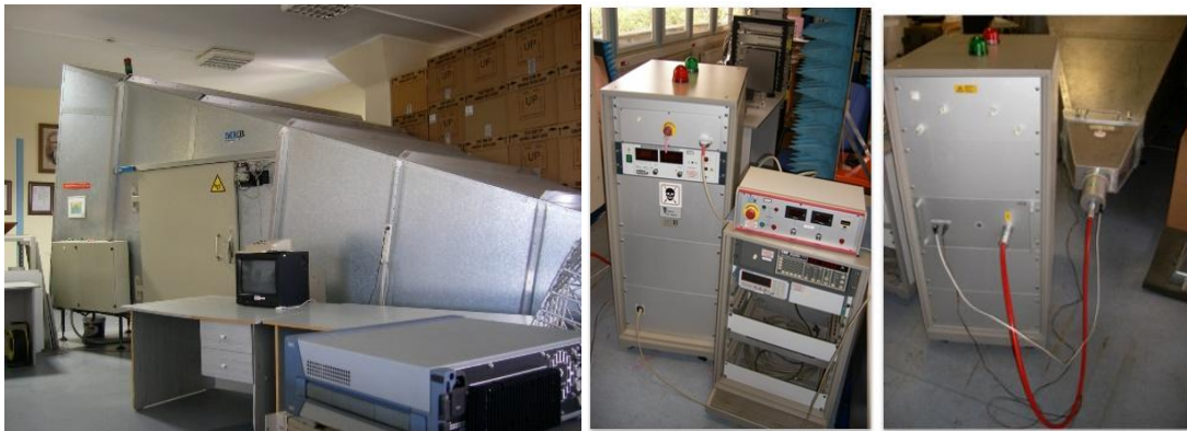
Figure 4: Measurement setup of GTEM, EMP generator and Control unit
