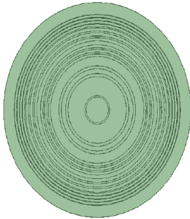
Figure 4: Layered Cylindrical Luneburg lens with partial filling of Dielectric with concentric grooves
