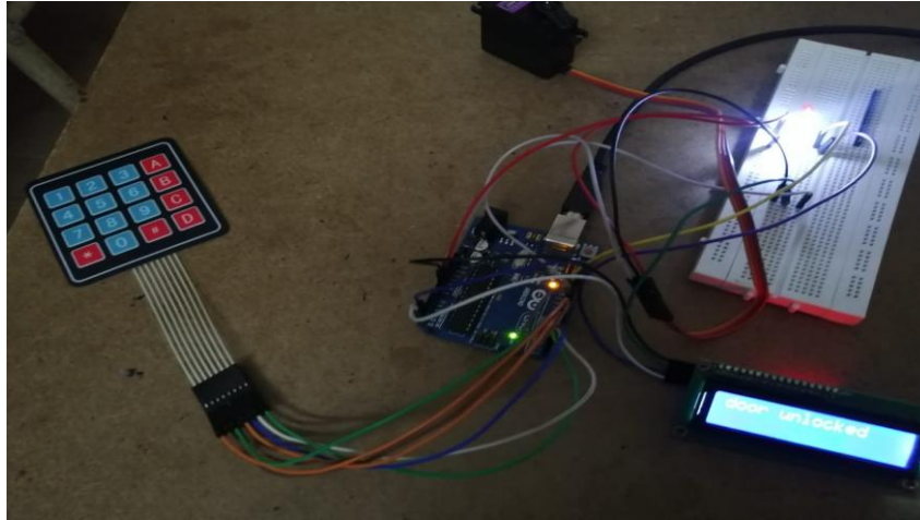
fig: working model of door lock system
