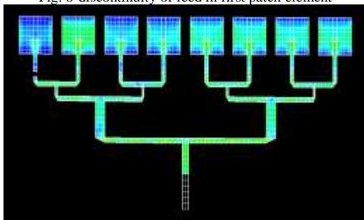
Fig. 7- current distribution in single fault
