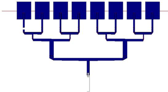
Fig. 6-discontinuity of feed in first patch element
