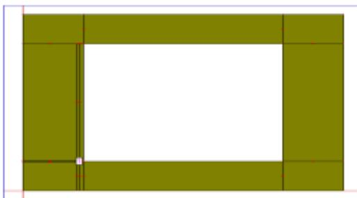
Fig. 7: Proposed Geometry of rectangular ring slot antenna on IE3D
