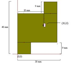
Fig.3 Geometry of RMSA with two slots
