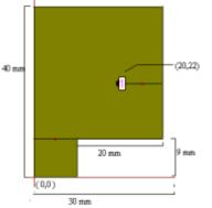
Fig.2. Geometry of RMSA with one slot.
