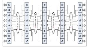
Figure 5. Four stage pipeline 1D-DCT.
