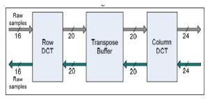
Figure 3 Architecture of 2-D DCT
