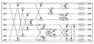
Figure 4. Architecture of 1-D DCT
