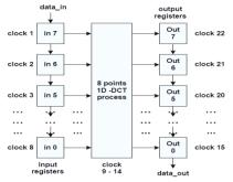
Figure 7. 1-D DCT with pipelining
