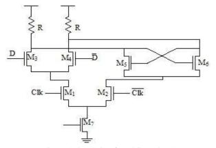
Fig. 2. Schematic of an SCL D latch.
