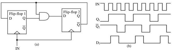
Fig. 6. (a) Divide by 3 prescaler and (b) timing diagram.
