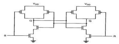
Fig. 11. SR latch designed by CMOS logic.
