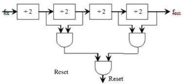
Fig. 9. The designed circuit for program counter.
