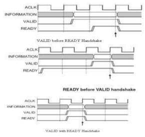
Figure3. Waveforms for handshaking mechanism
