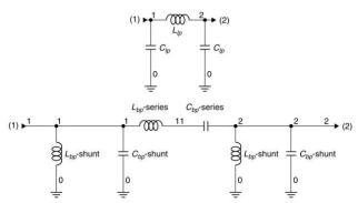
Figure 1. Bandpass filter prototype starting with low pass filter
