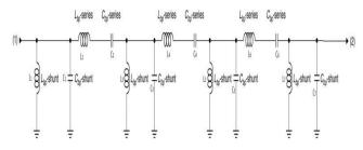
Figure 2. Bandpass filter with N=7
