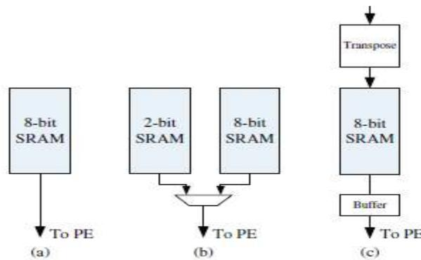
Fig. 7. SA memory arrangement (a) mem8 (b) mem28, and (c) mem8pre.
