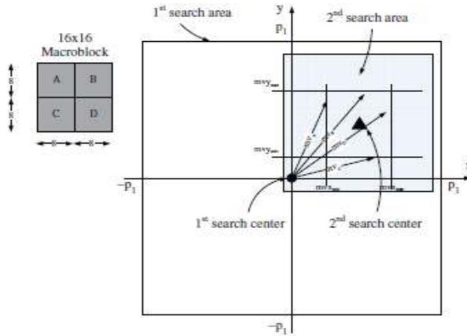
Fig. 3. Defining the second search area for the proposed two-step algorithm.
