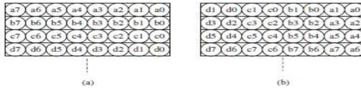
Fig. 8. Storing 8-bit pixel in 8-bit memory: (a) conventional arrangement and (b) mem8pre.
