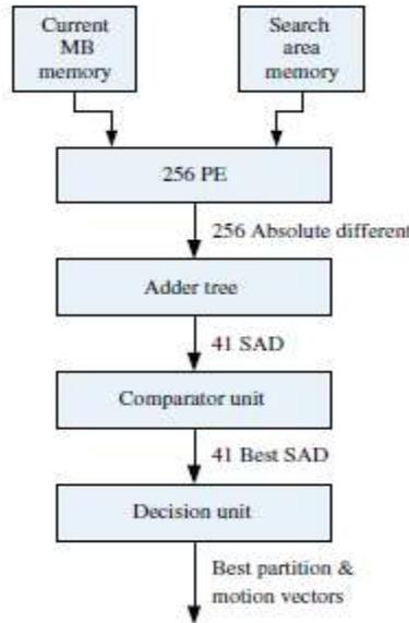
Fig. 4. Me\_sad block diagram.
