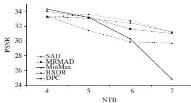
Fig. 2. Average PSNR versus NTB for different block matching criteria using  $8 \times 8$  block size (50 Foreman frame sequences, QCIF@30frames/s, search range,  $p = [-8, 7]$ ).
