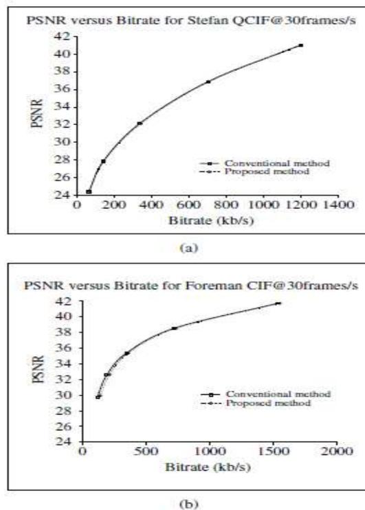
Fig. 9. PSNR versus bitrate using the proposed two-step method for (a) QCIF@ 30 frames/s,  $p = [-8, 7]$  and (b) CIF@30 frames/s,  $p = [-16, 15]$ .
