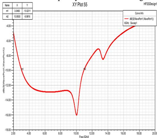
Fig. Simulated Return loss of designed antenna
