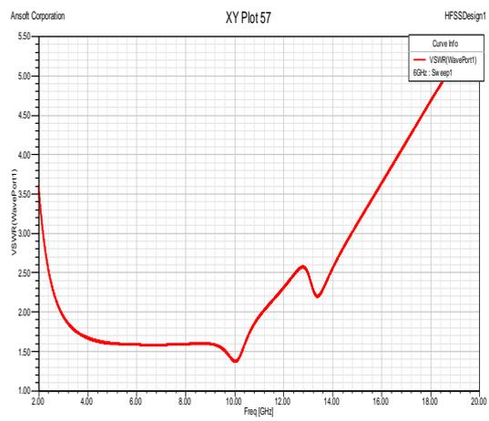
Fig. Simulated VSWR of designed antenna
