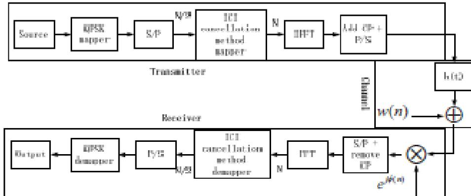
Fig.1 Diagram of OFDM system using the proposed method
