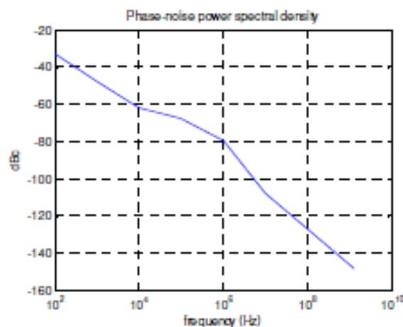
Fig. 3. Phase noise model in the simulation
