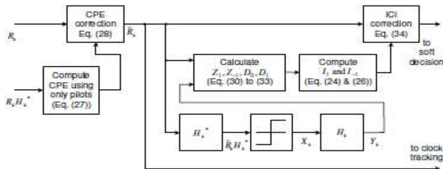
Fig. 2. Details of the CPE and ICI compensation in Fig. 1.
