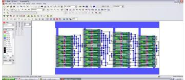
Figure 8. Full Custom Layout of 45nm 8-bit Flash ADC
