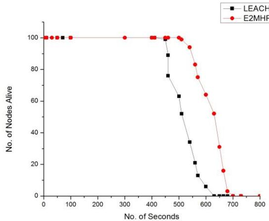
Fig. 2 Comparison Of Network Lifetime
