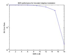
Figure 3. BER Performance of Uncoded AOFDM with BPSK, QPSK,QAM
