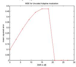
Figure 4. Mean Square Error of Uncoded OFDM with BPSK, QPSK, QAM
