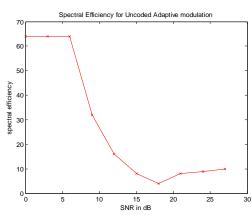
Figure 6. Spectral efficiency of Uncoded OFDM with BPSK, QPSK,QAM
