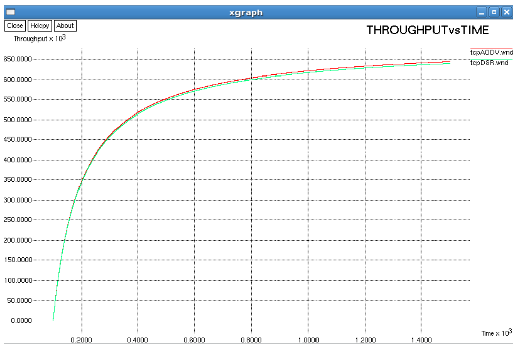
Fig. 6: Comparison of Throughput for reactive routing protocols AODV and DSR
