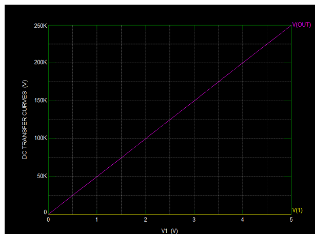
Fig 3 : High Sense Amplifier- Input Signal Vs Output Signal
