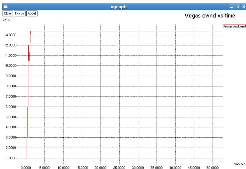
Figure 4 cwnd vs. Time for TCP Vegas
