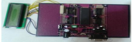
Fig. 8: Microcontroller-89c52 Board
