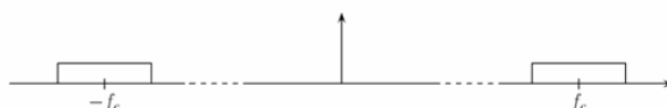
Fig. 1: Spectrum of Transmitted Pass band Signal But the channel may have a completely non-uniform spectrum, as can be represented by Fig. 2.
