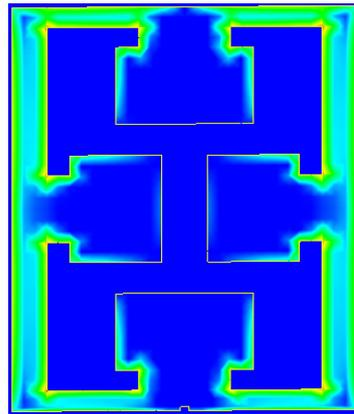
Fig-(3.11) current distribution of final patch shape
