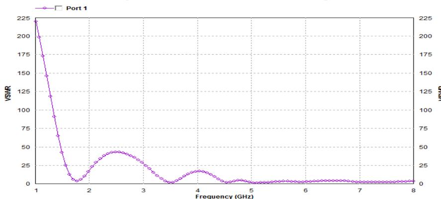
(Fig-(3.2): VSWR curve of base shaped antenna)
