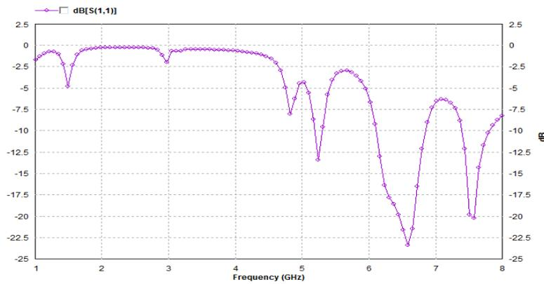
(Fig-(3.7) Return loss curve of 1 iteration)
