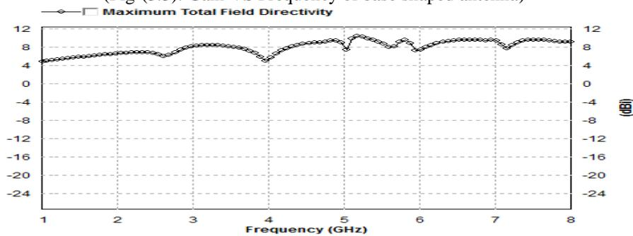
( Fig-(3.4) : Directivity VS Frequency graph of base shaped antenna)
