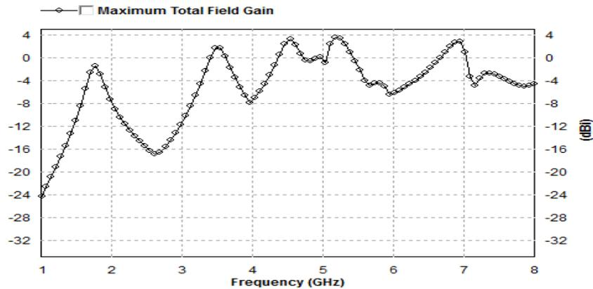
(Fig-(3.3): Gain VS Frequency of base shaped antenna)
