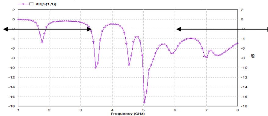
(Fig-(3.1): Return loss curve of base shape)
