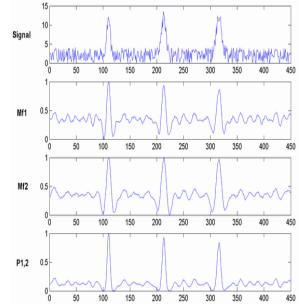
Fig. 5 Anisotropic filtering and scale production: Mf1 and Mf2 are the responses at two different scales, P1,P2 is their production According to our experience, the palm vein widths in our infrared images vary from 10 pixels to 20 pixels that corresponding to Gaussian with standard derivation from 1.2 to 2.4. In order to produce strong filter responses, the standard derivation of the anisotropic filters must be similar to the standard derivation of veins.
