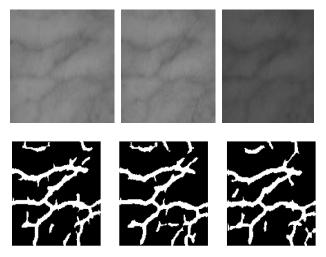
Fig. 8. Images of a palm captured at different times, where the image quality is good. The first row shows the images captured by our device. The second row shows the corresponding vessel extraction results. The recognition performance is shown in Figure 11 using ROC curve. We achieved 98.8% recognition rate where the false acceptance rate is 5.5%. Most of the false recognitions were caused by the images of poor quality.
