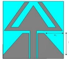
Fig.2.1: Structure of monopole antenna varying the parameters  $P_1, P_2$
