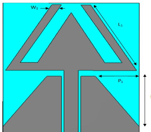
Fig.2.5: Structure of monopole antenna varying the parameters  $L_1$
