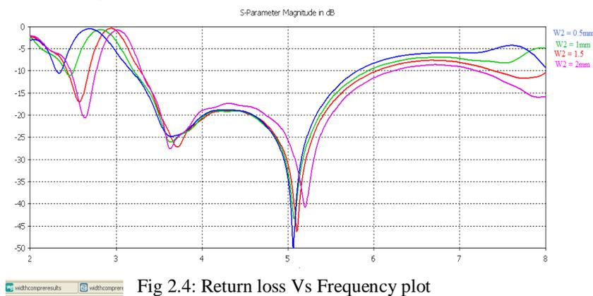
Fig 2.4: Return loss Vs Frequency plot
