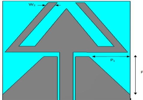
Fig.2.3: Structure of monopole antenna varying the parameters  $W_2$
