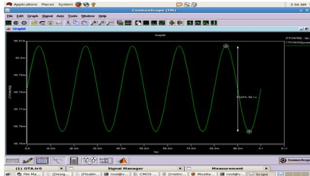
Fig.5 Hspicesimulation of Simple Differential OTA
