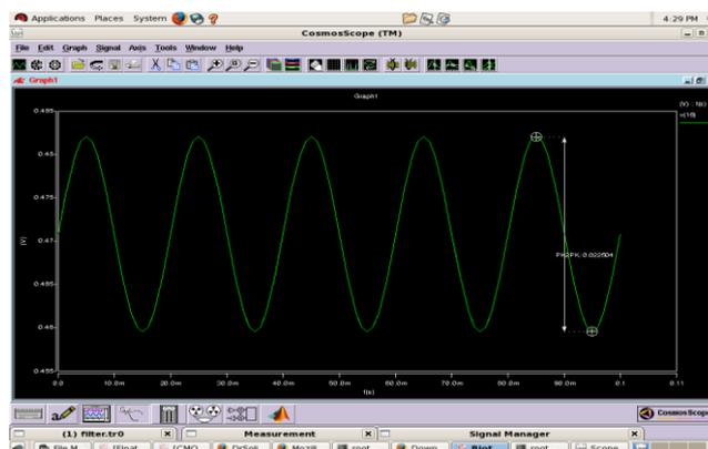
Fig.7Hspice Simulation of OTA-C filter design
