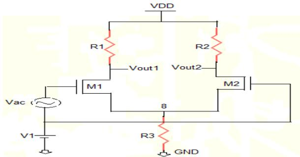
Fig. 1 Differential Amplifier with source degeneration
