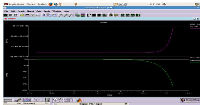
Fig.6 Frequency response with the cutoff frequency 300Hz and phase
