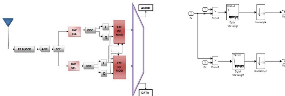
Fig:2. Block Diagram of proposed for Multi-channel Monitoring Receiver, Fig: 3 DDC of Single Channel
