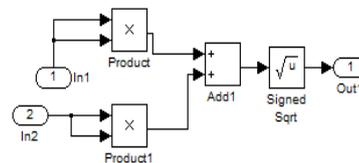
Fig:5. AM Demodulator algorithm.
