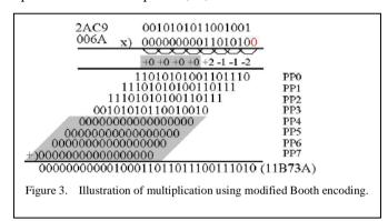
Fig-3 shows a computing example of Booth, multiplying two numbers, "2AC9" and "006A". The shadow denotes that the numbers in this part of Booth multiplication are all zero so that this part of the computations can be neglected. Saving those computations can significantly reduce the power consumption caused by the transient signals.
