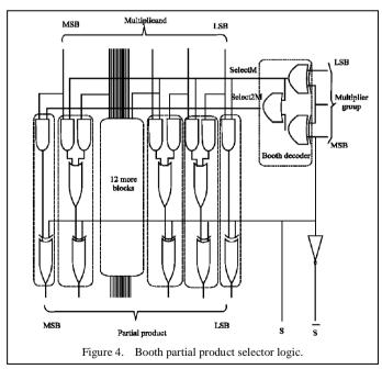
According to the analysis of the multiplication shown in fig-3, we propose the SPST-equipped modified-Booth encoder, which is controlled by a detection unit. The detection unit has one of the two operands as its input to decide whether the Booth encoder calculates redundant computations.
